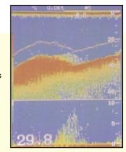
The bottom is displayed as a straight line on the lower part of the screen, regardless of bottom contour. This mode is useful for detection of fish close to or on the bottom.
